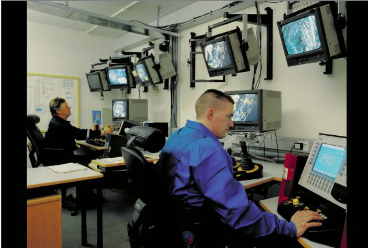
Mine control room, Zinkgruvan, Sweden, including automated drill rigs. Photograph courtesy of Atlas Copco
