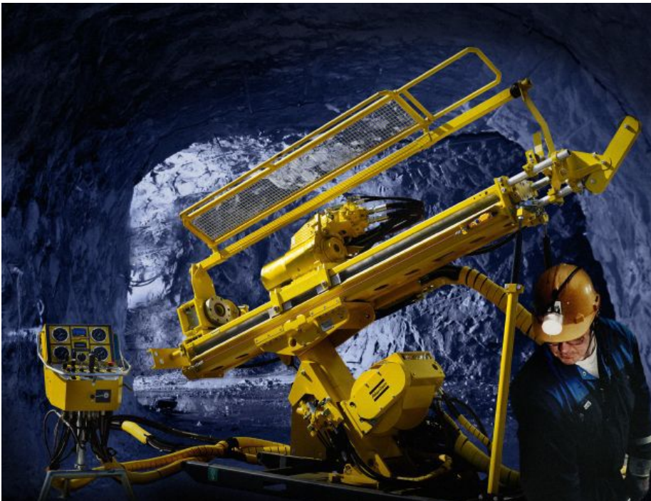
Underground coring rig, complete with MWD, allows remote operation from surface. Photograph courtesy of Atlas Copco
