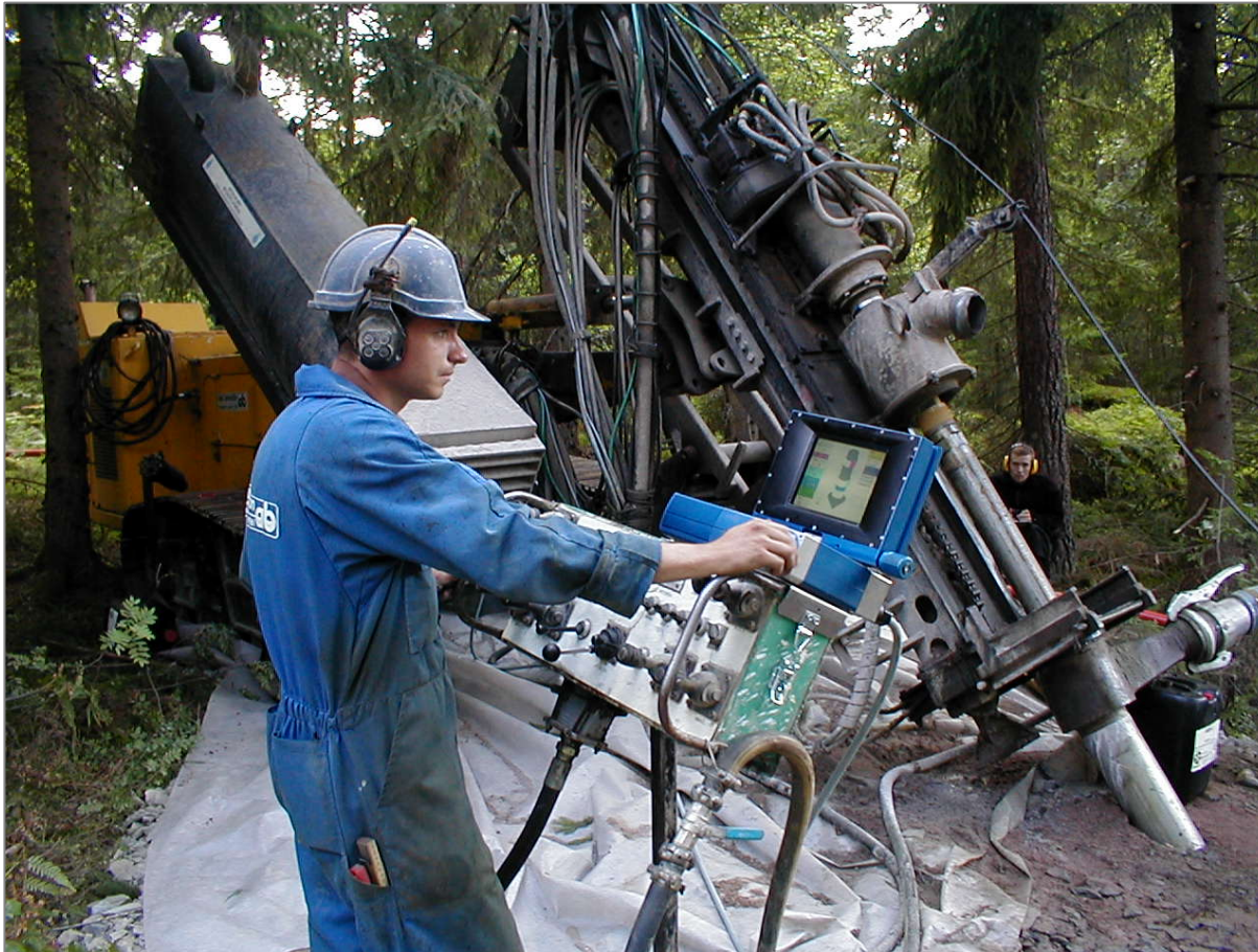
Rotary coring supplemented by MWD for geotechnical investigations for potential nuclear waste depository sites, Sweden. Photograph courtesy of Environmental Mechanics, SE
