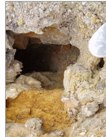
Open joint from Lincolnshire Limestone, Ketton Quarry. Photo graph courtesy of P. del Strother
