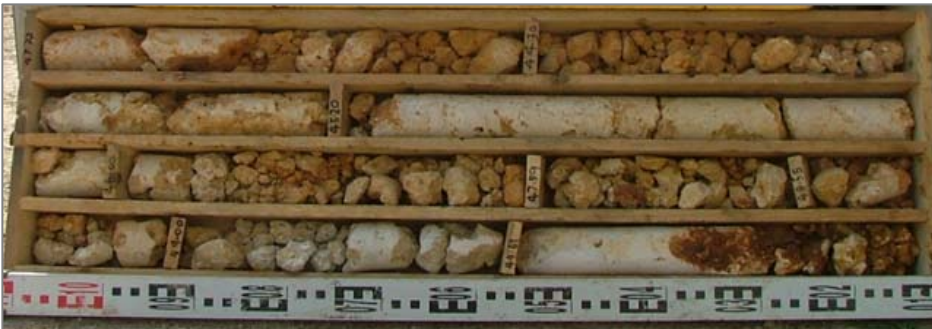
HQ core recovery voided Limestone
